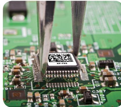
Barcode labels that may be exposed to heat, static electricity or solder - such as those used on printed circuit boards - undergo a highly sophisticated manufacturing process using specialized materials that help to reduce the occurrence of electrostatic discharge.
