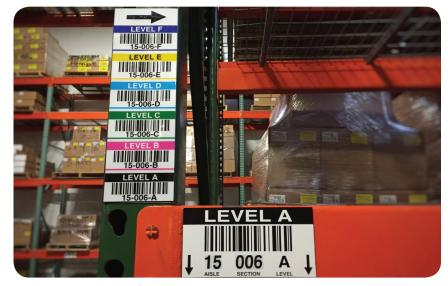
Vertical upright labels eliminate the need for long-range scanning, minimize potential confusion and errors, and ensure more efficient operations
