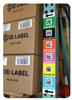
A vertical location label is a grouping of barcodes—often color coded by level that contains specific information for each level of racking within a bay.
