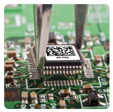
Sensitive electronic components can be significantly damaged by electrostatic discharges that can occur during the manufacturing process and throughout a device's useful life.
