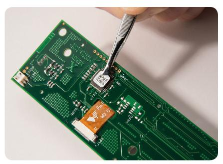
Polyimide barcode labels help to reduce the occurrence of electrostatic discharge in sensitive electronic components.
